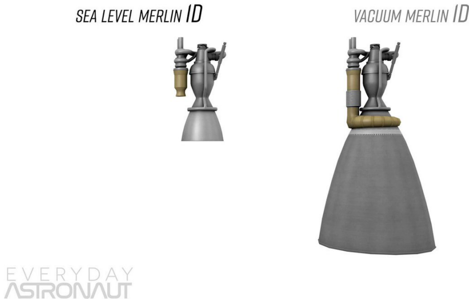
Figure 4.7: First and Second Stage Size Comparison from Everyday Astronaut
